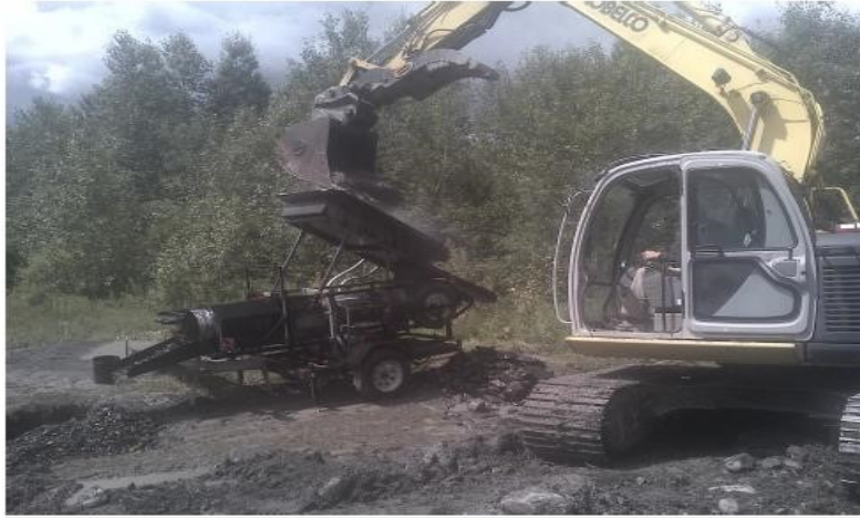
Figure 19: A view of the mobile washing plant being loaded by a small excavator.
