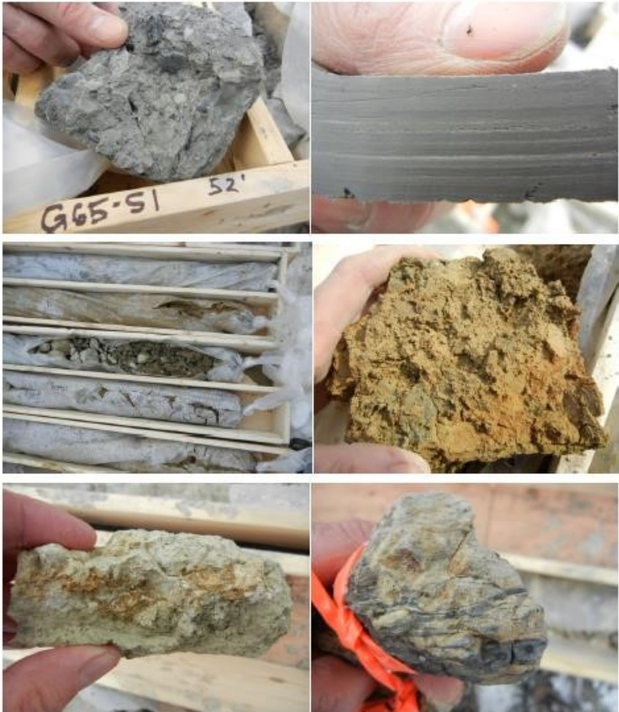
Figure 26: Pictures of Sedimentary units. From top left to lower right: Detail of the grey silty diamicton (Unit 1); finely laminated silt and fine sand (Unit 2); cores and details of the brown clayey diamicton (Unit 3); and brownish beige alterite (Unit 4) and its underlying bedrock.
