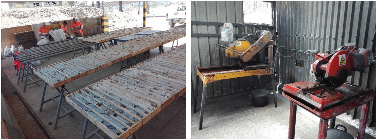
Figure 11.5 –Logging and Sawing of Drill Core (Atalaya 2018)
