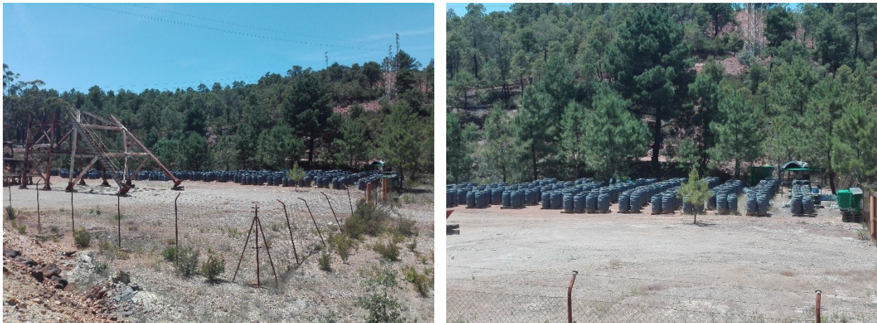
Figure 11.3 - Storage Yard for RC Cuttings (Atalaya 2018)
