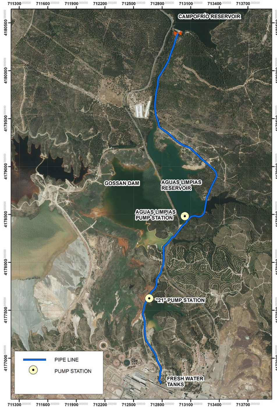
Figure 18.1 – Fresh Water Distribution System (Atalaya 2018)
