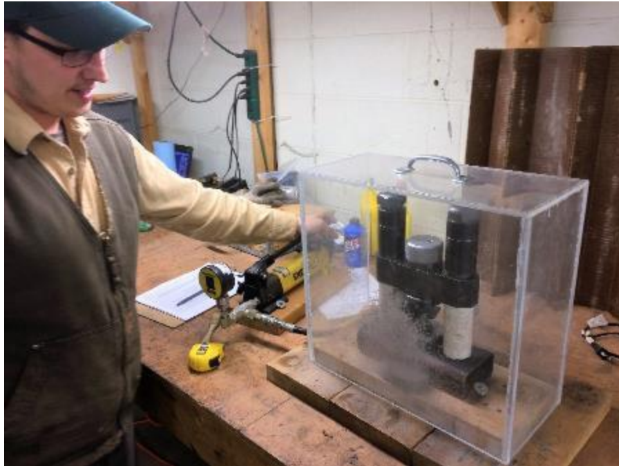
Figure 10.6: Point Load Testing (Bemek Rock tester)
