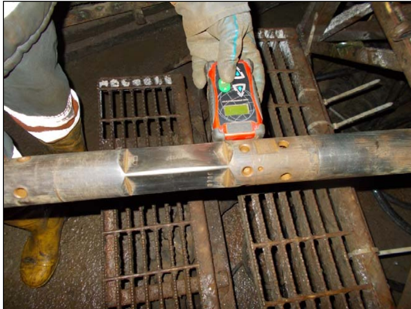
Figure 11. Process of core orientation at underground drill site by a driller using Orifinder controller. (DPMC, 2015).
