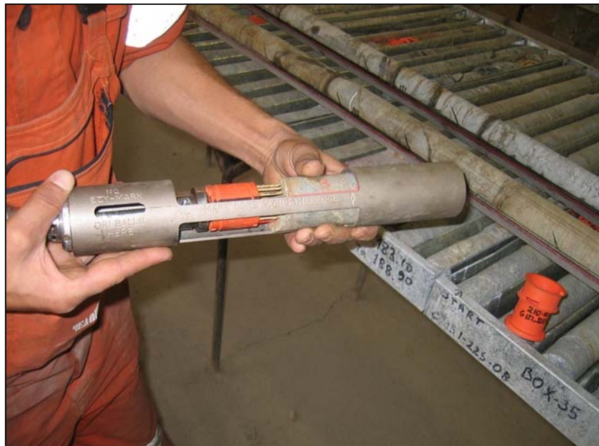
Figure 10. Check on core orientation by Geotechnician using the Ezy-Mark™ system. (DPMC, 2013)
