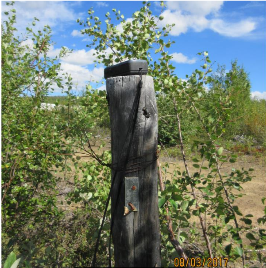
Figure 10.2 Typical collar marking for Underworld drill holes at White Gold
