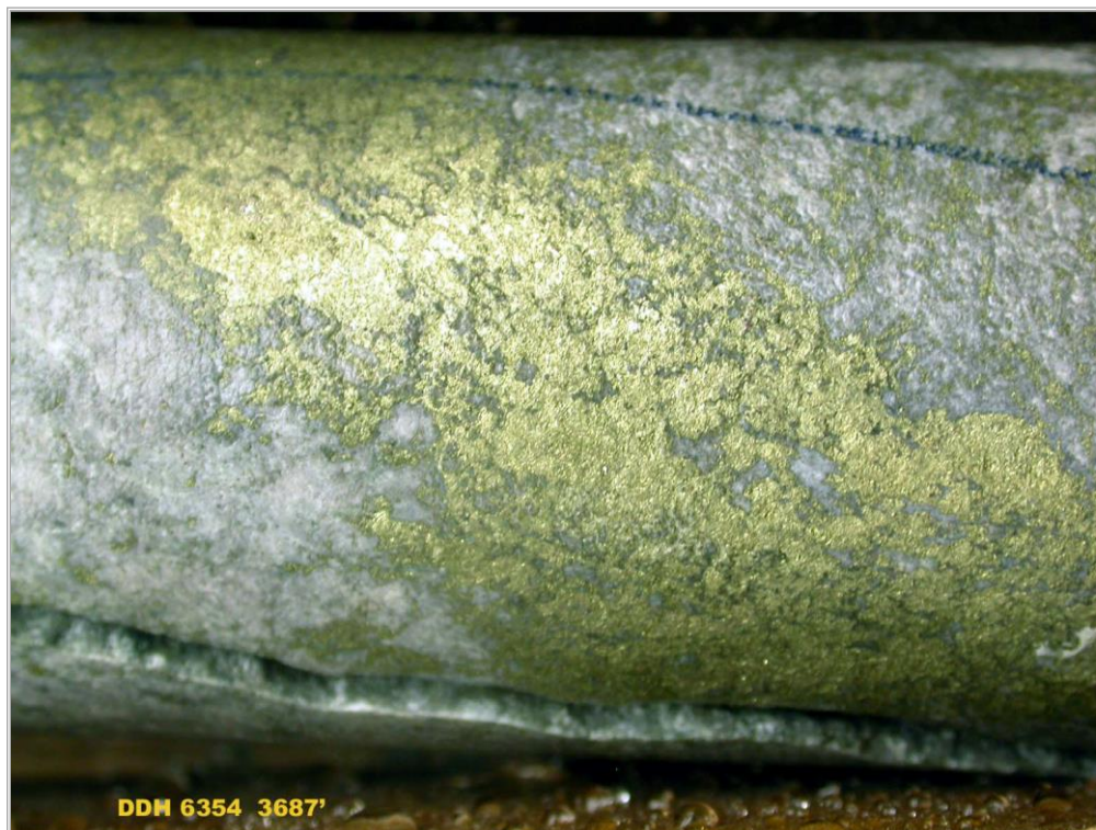
Figure 7.5-1 Drill Core Photograph Showing Chalcopyrite Mineralization
