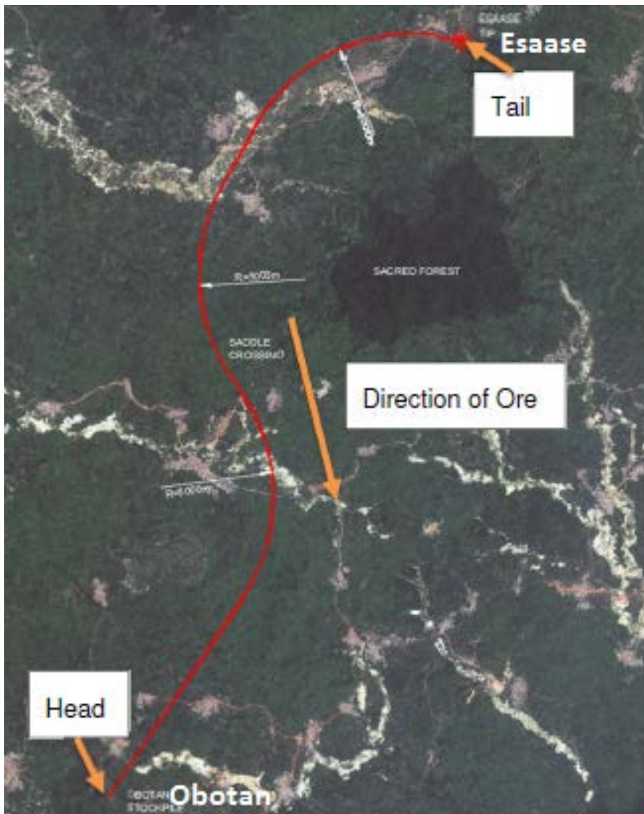
Figure 18-4: Overland Conveyor Route (source: ELB 2017)
