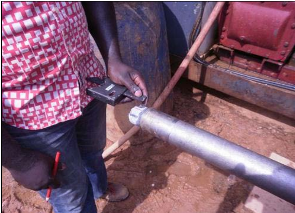
Figure 10-11: Core Orientation Procedures using a Reflex ACT II System (Source: Spiers 2011)
