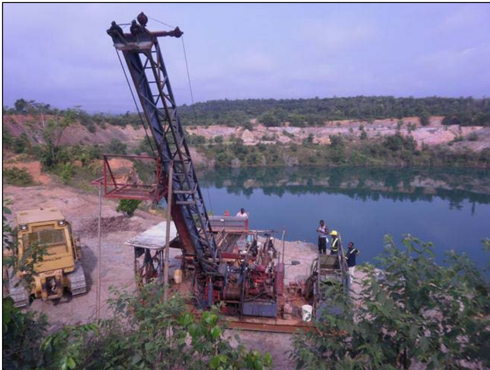
Figure 10-9: Hole NKR11-040 Drilling on the SE side of the Nkran Open Pit (2011) (Source: Spiers 2011)
