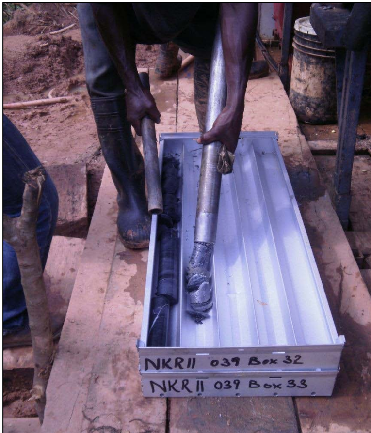
Figure 10-10: Laying Core out into Pre-marked Trays (Source : Spiers, 2011)
