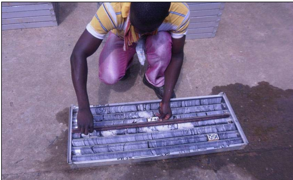
Figure 10-14: Marking up Core prior to Cutting (Source: Spiers 2011)
