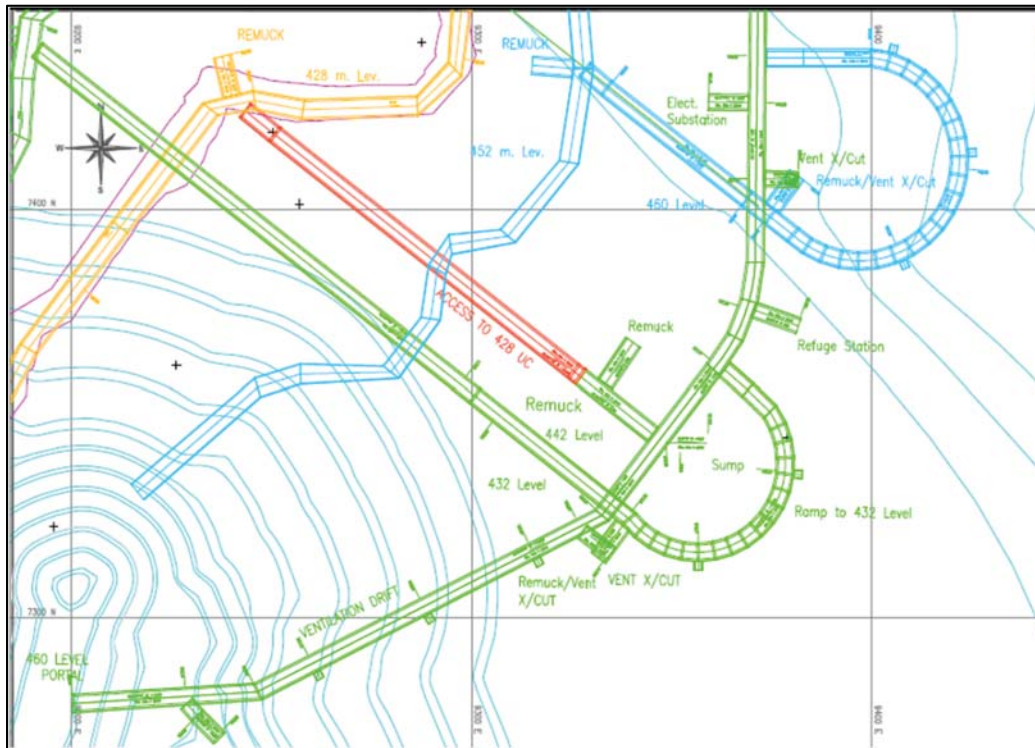
Figure 16-6: Plan View of Ramp from Surface to 468 Level
