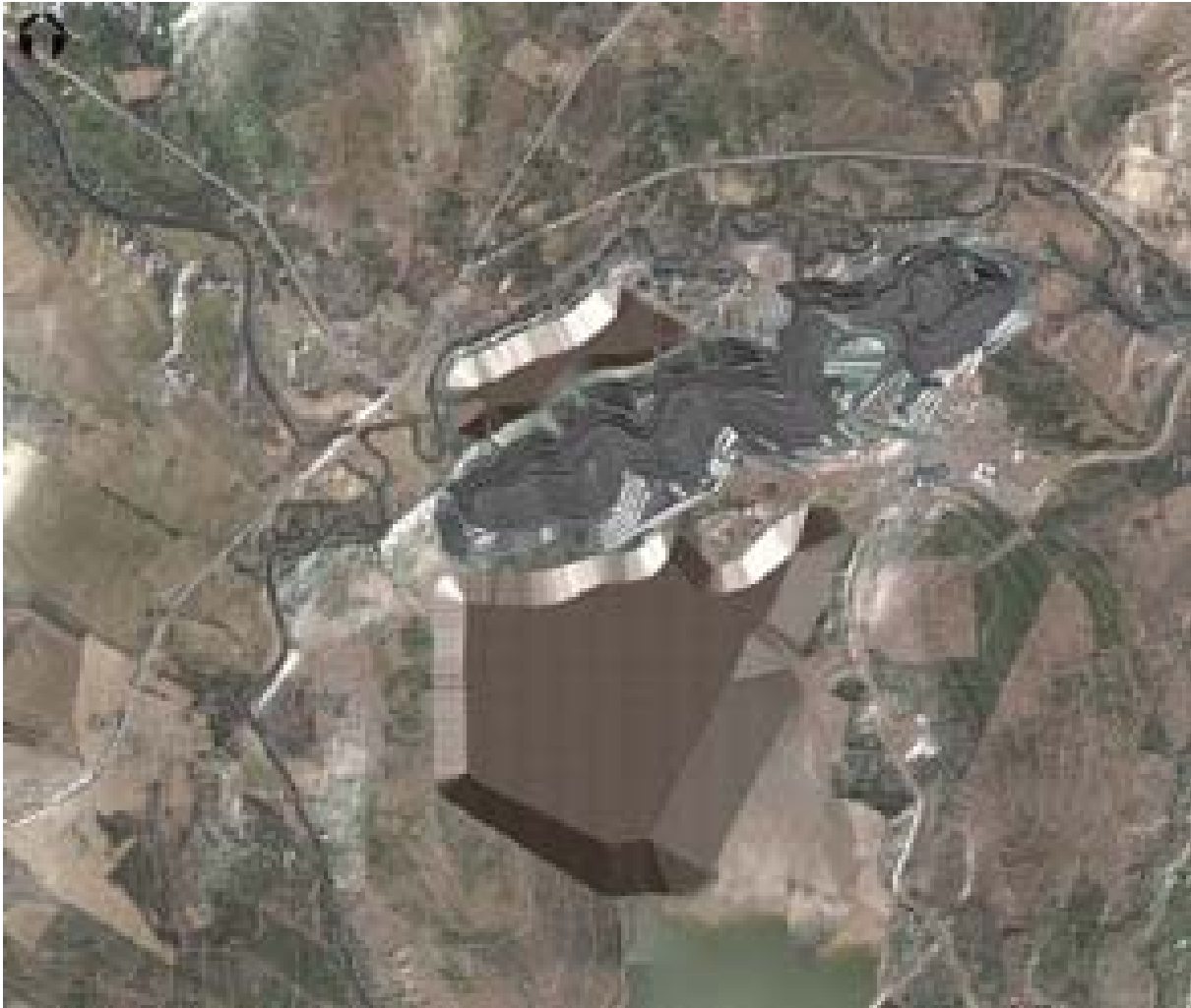
Figure 16-3: Waste Pile Locations
