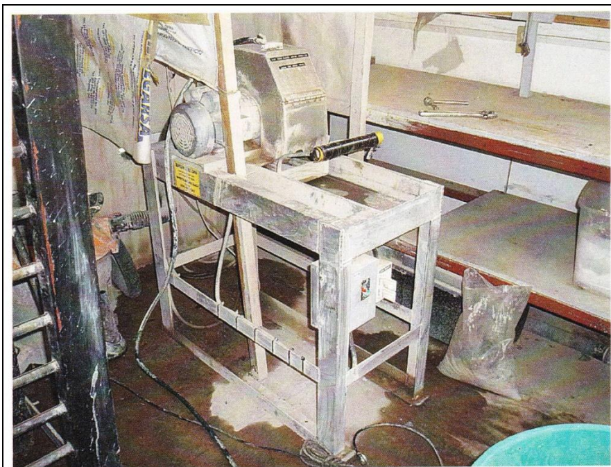
Core splitting facilities – Diamond saw (B. Solano, 2009)
