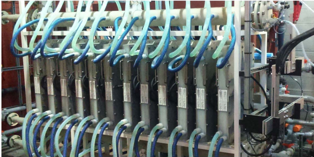
Production-scale vanadium electrolyte equipment
