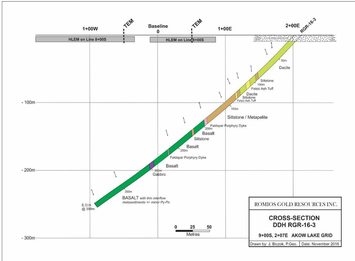
Figure 9: Cross section of DDH RGR-16-3
