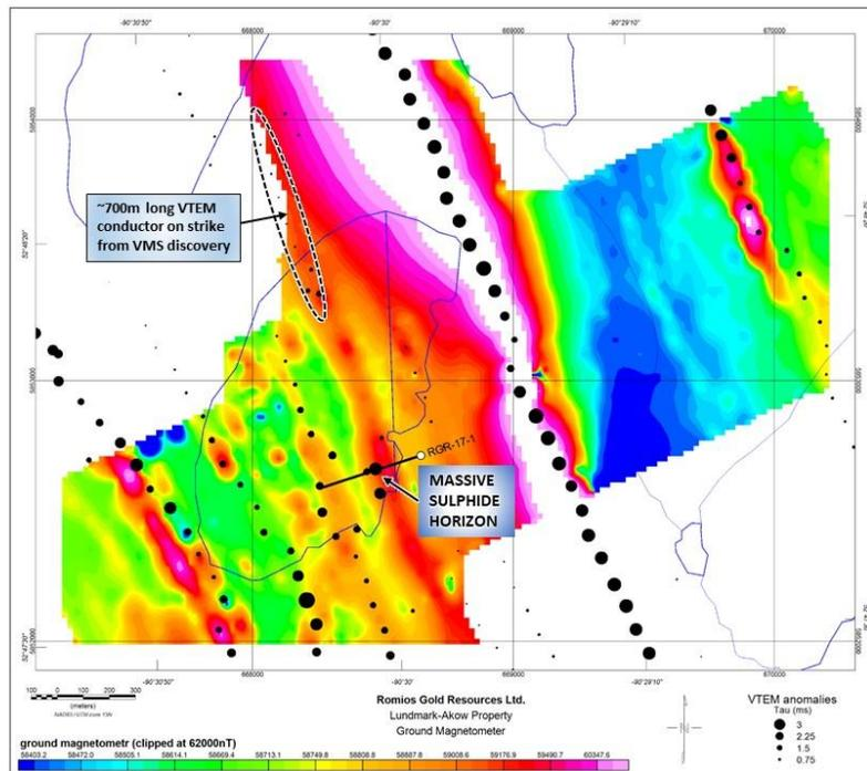
Figure 20: VTEM conductors overlain on ground magnetics, Atim Lake North area
