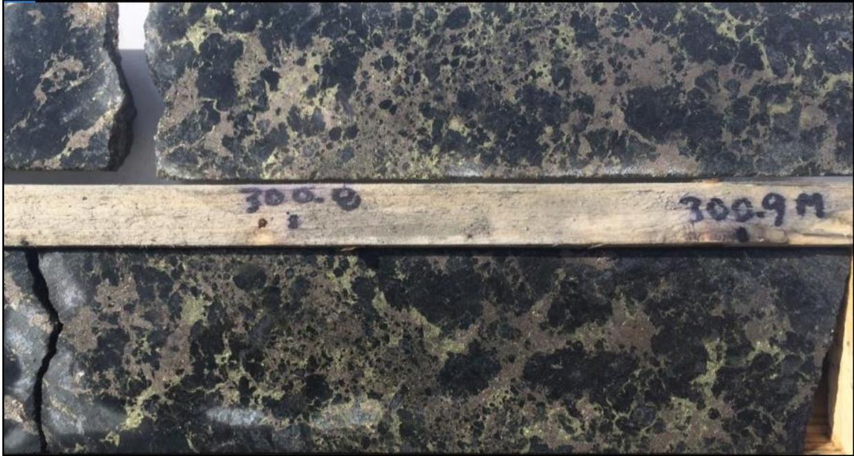
**Plate 1: High grade portions of the massive sulphide horizon**
