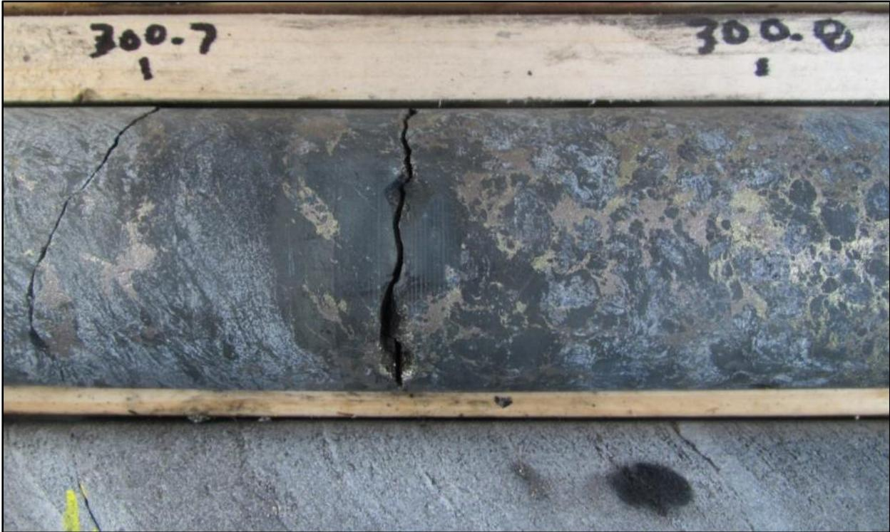
**Plate 3: Tourmalinite-rich section of the massive sulphide horizon.**
