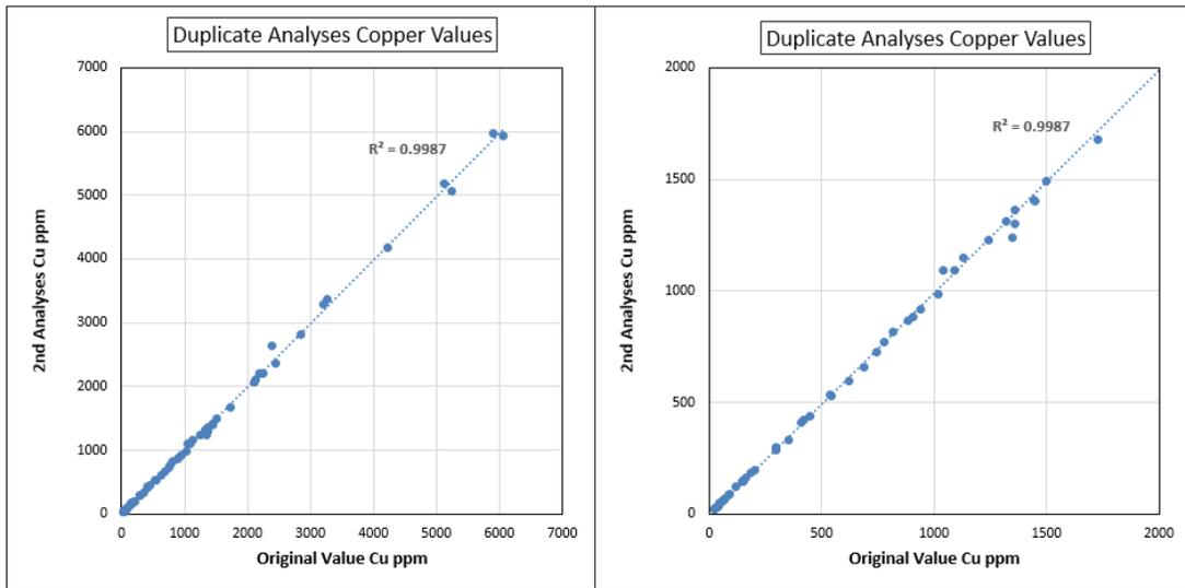
The correlation between results from the original and repeat copper analyses is excellent with a correlation coefficient of 0.9987. There is no obvious bias evident in either graph towards a higher or lower value in the repeat analyses with respect to the overall amount of copper. The individual results are listed below in Table 19.
