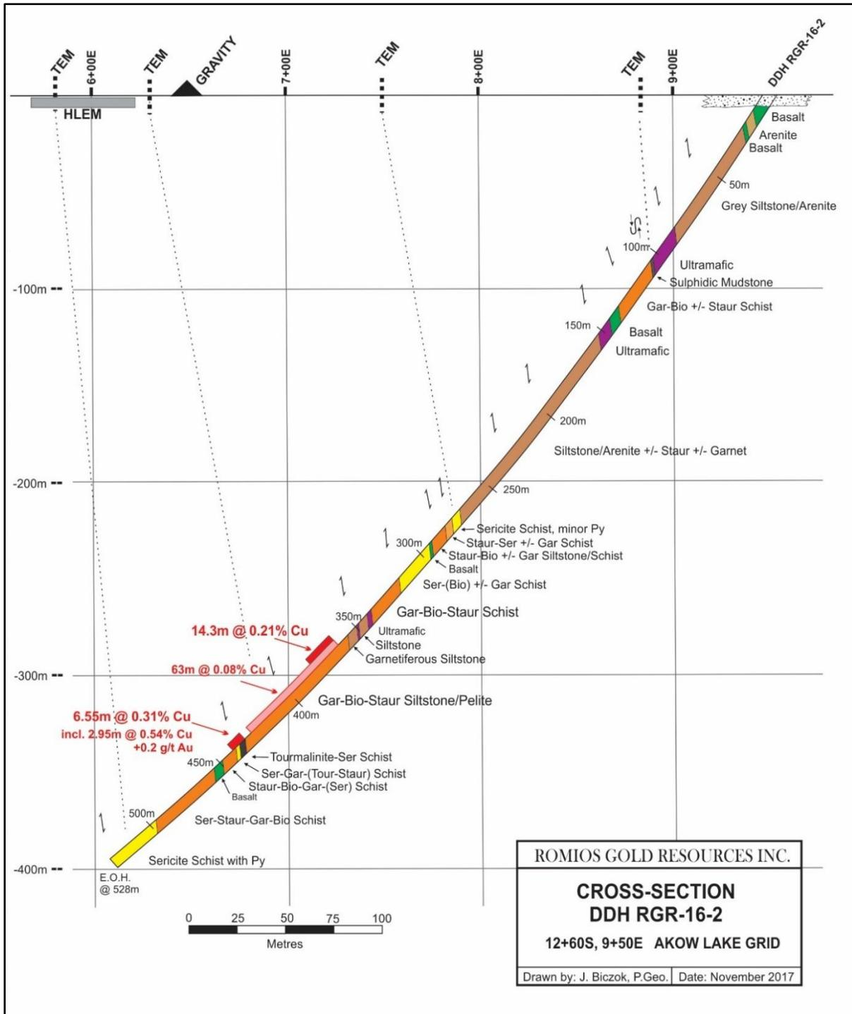
Figure 8: Cross section of DDH RGR-16-2
