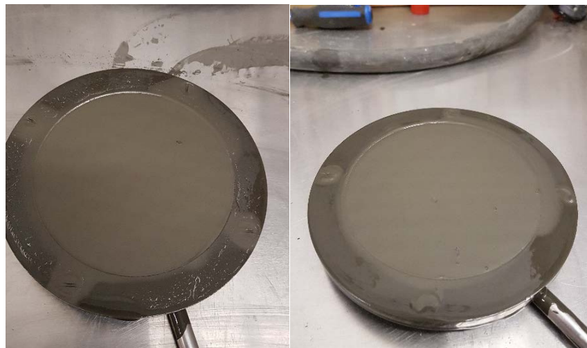
Figure 13-57: 50/50 PFT/PCT vacuum filtration cakes – 53.5% w/w slurry feed (left) and 60% w/w (right)
