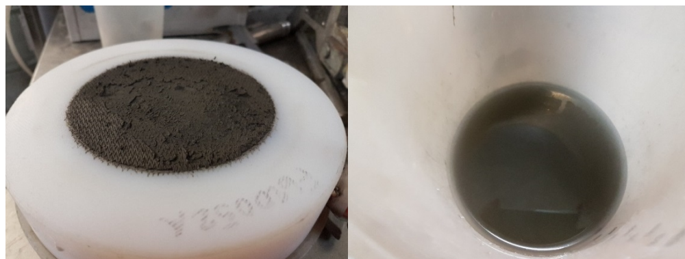
Figure 13-56: 50/50 PFT/PCT pressure filter cake (left) and filtrate (right)
