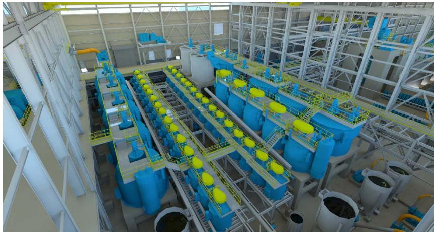
Figure 17-6: Configuration of the flotation circuit – close-up on copper and zinc circuits
