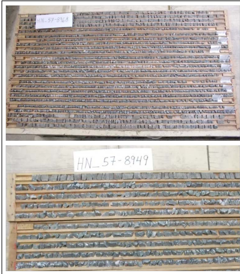
Figure 12-1: Photographs showing general presentation of quarter-split core after resampling
