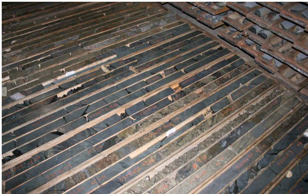
Figure 12-18: Half-core witness samples from mineralized zones
