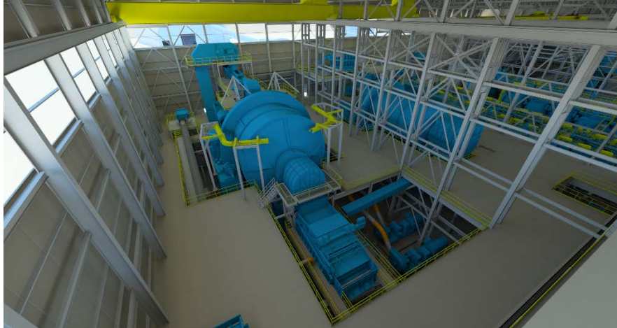
Figure 17-5: 3D model arrangement of the SAG mill and ball mill circuit
