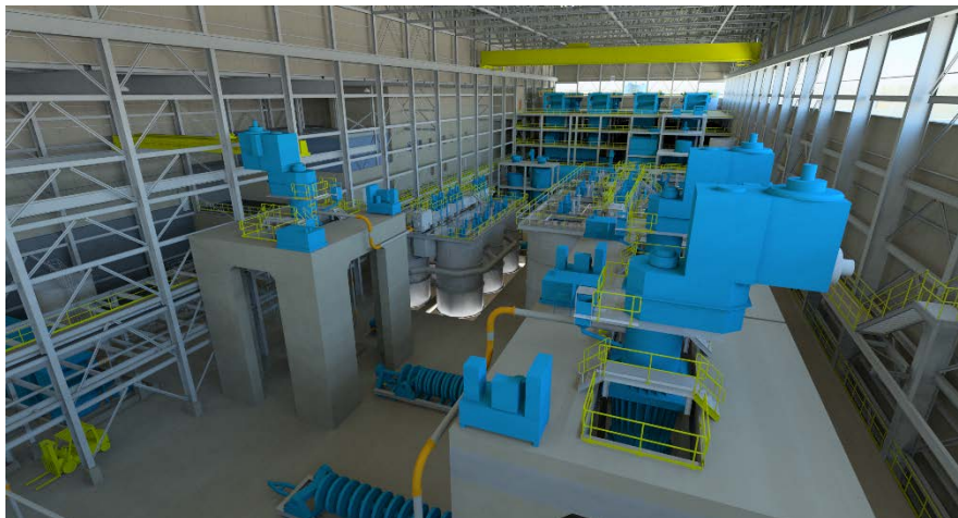
Figure 17-10: Configuration of the pyrite concentrate regrinding circuit
