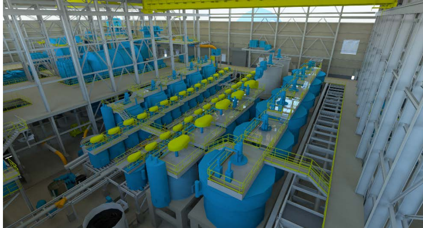
Figure 17-7: Configuration of the flotation circuit – close-up on the pyrite circuit
