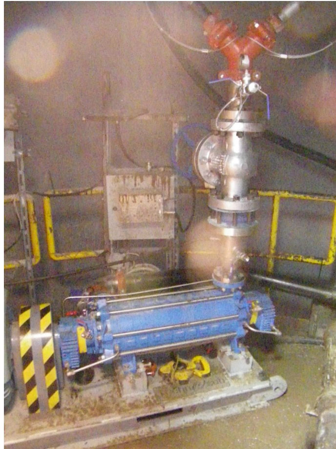
Figure 16-13: Typical booster pump installed on a Galloway
