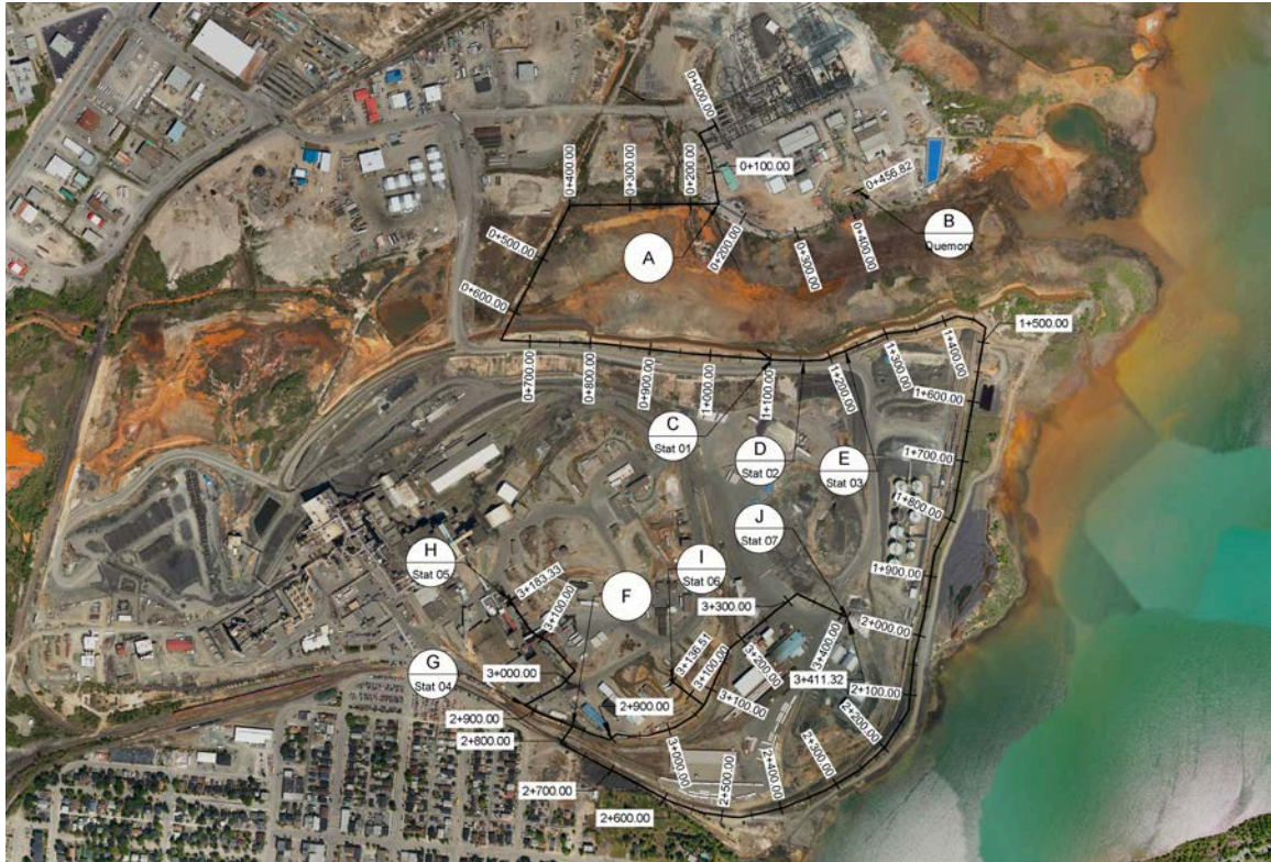
Figure 16-70: Proposed surface slurry pipeline on Horne property
