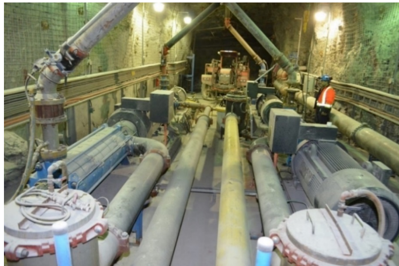
Figure 16-27: Typical underground multistage pump dewatering station
