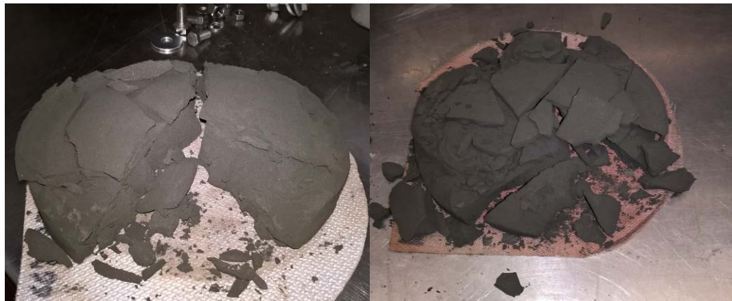
Figure 13-58: Filtered cake of 100% PFT and 50/50 PCT/PFT
