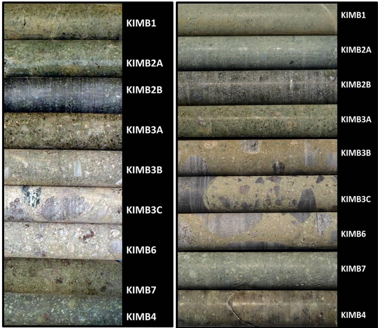
Figure 7-9. Drill core photographs of the Kelvin kimberlite units in the South (left) and North (right) Limbs
