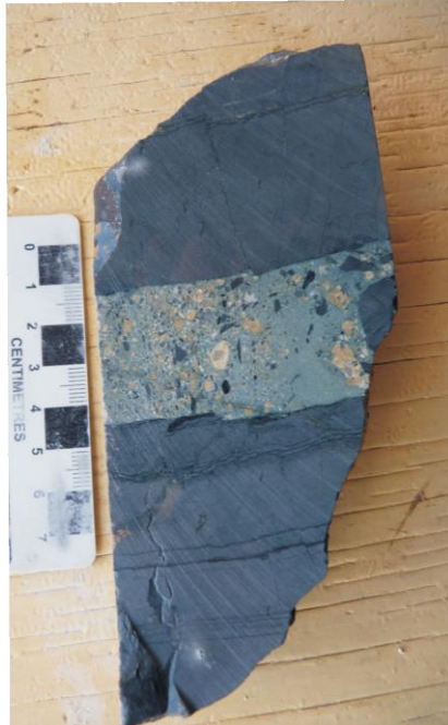
Figure 7-10: Dyke of Tuff in Basement Rocks from Hole CGA-116. (Golden Arrow, 2015)
