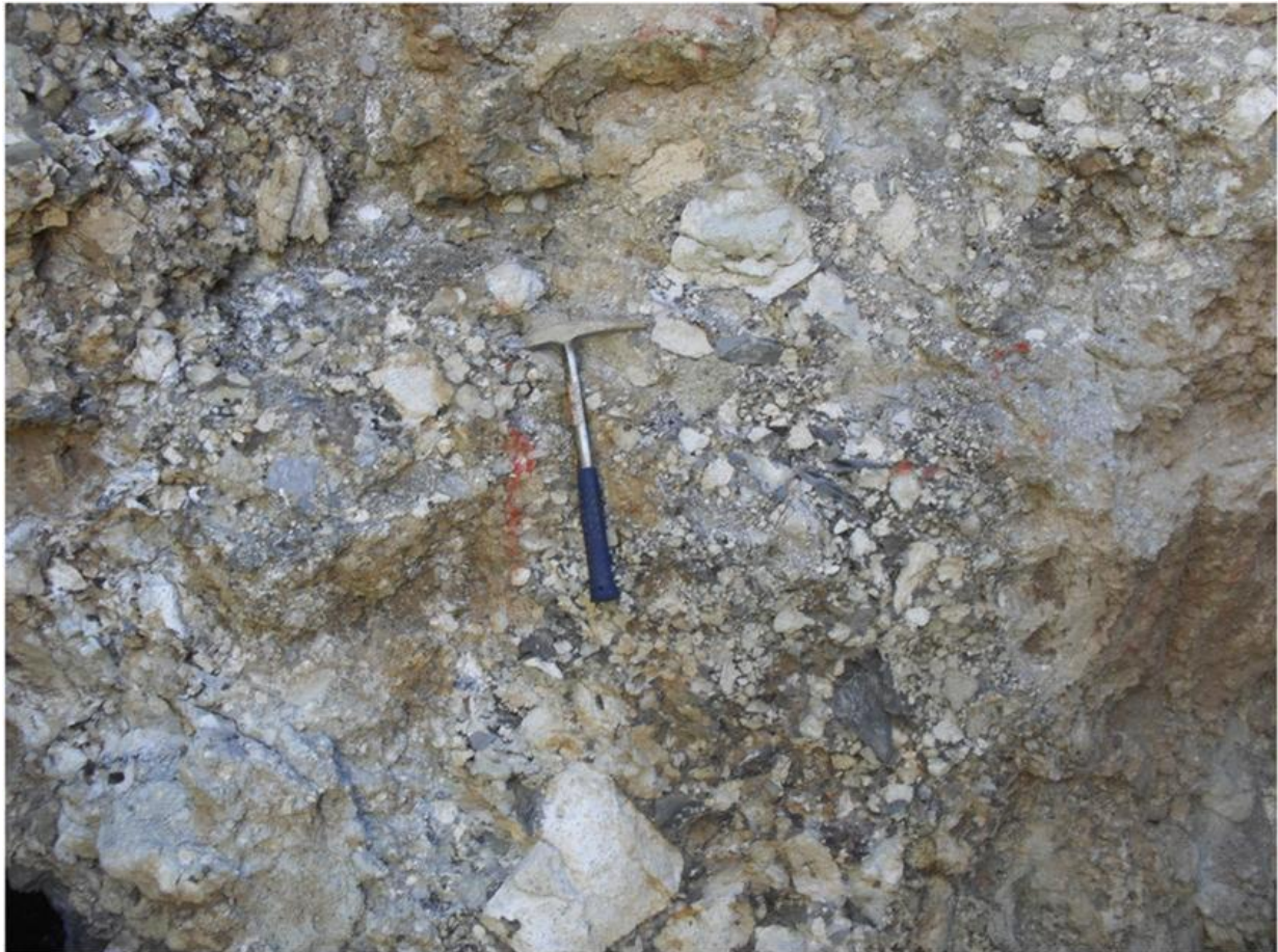
Figure 7-9: Coarse Grained Clast-Supported Breccia at Socavon del Diablo. Mineralization Infilling Matrix and Open Spaces. (Golden Arrow 2013)
