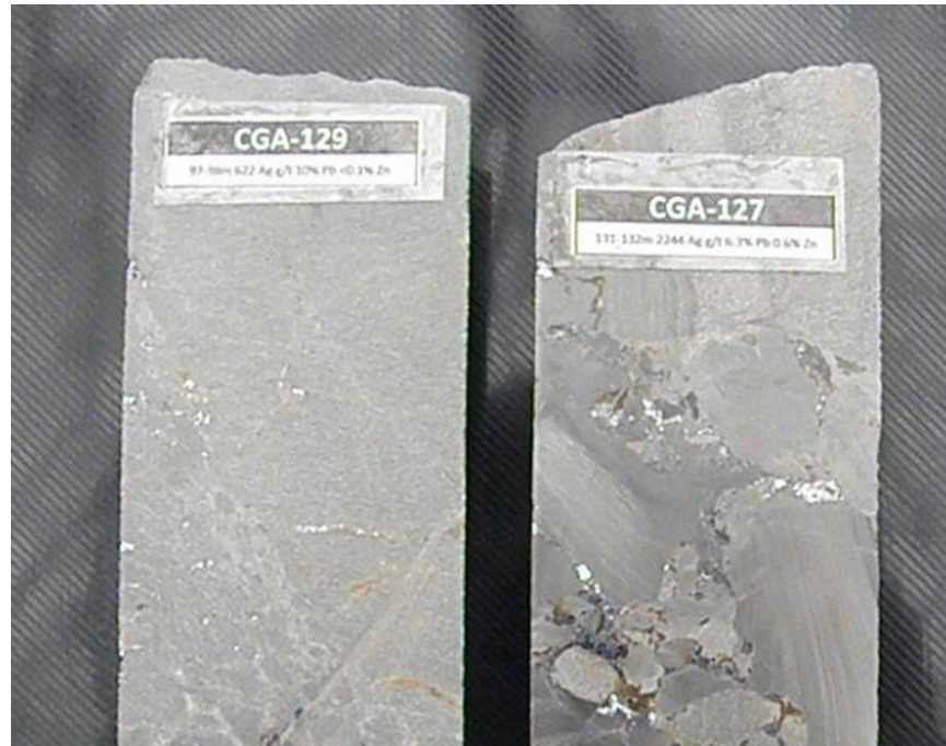
Figure 7-17: Typical Fracture Filling and Breccia Cement Mineralization in Basement. Galena, Sphalerite and Siderite Infilling. (Golden Arrow, 2014).
