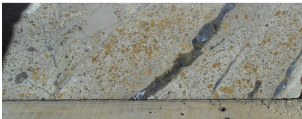
Figure 7-19: Galena-Ag Veinlets in Dacite. (Golden Arrow, 2014)
