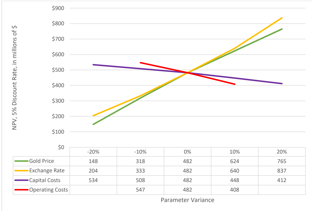
Figure 22-3 Sensitivity of Post-Tax NPV (5% Discount Rate) to various project inputs
