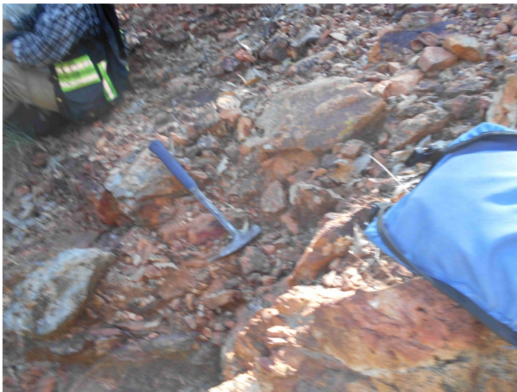
Photograph No. 12.1: Sample 2385, Silicified volcanics with hematite
