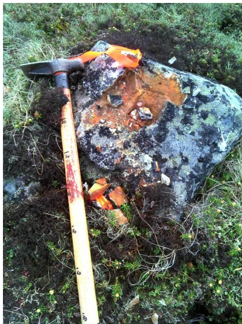
Photo 5: RB Zone quartz float found in 2015 (EFS), - sample # 660201 -38 grams/tonne gold (Cuttle, 2015)
