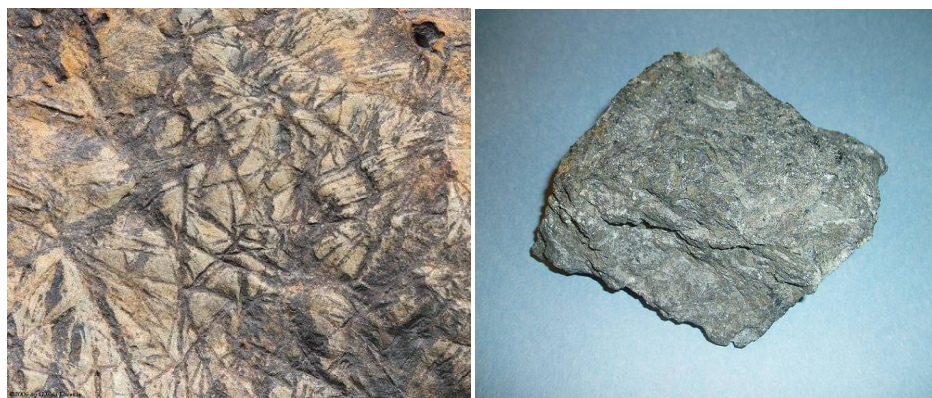
Photo 8: Typical spinifex texture in komatiite flow (L-weathered, R-fresh)
