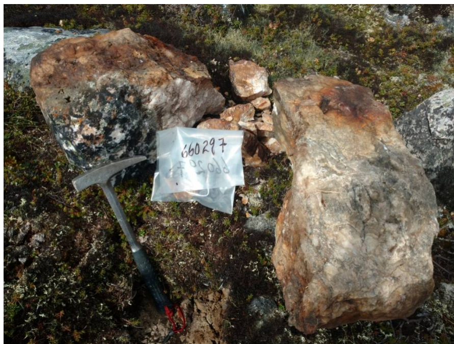
Photo 6: RIL Zone, quartz float found in 2016 (WML), approx. 90cm by 70cm in size. Sample # 660297 - 17.8 grams/tonne gold (Cuttle, 2016)
