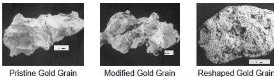
Photo 3: Typical gold grains from glacial till samples - Pristine, Modified and Reshaped (after ‘Overburden Drilling Ltd’ website)
