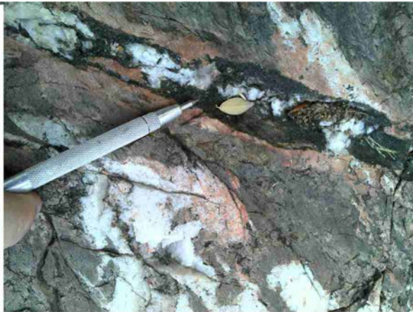
Fig. 9.12D Box mine area: quartz+biotite/chlorite vein cutting meta-sedimentary rock. note the K-feldspar selvage.
