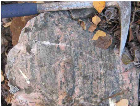
Fig. 9.12B Box mine area: K-feldspar altered biotite schist near contact with Box granite - partial "granitization".
