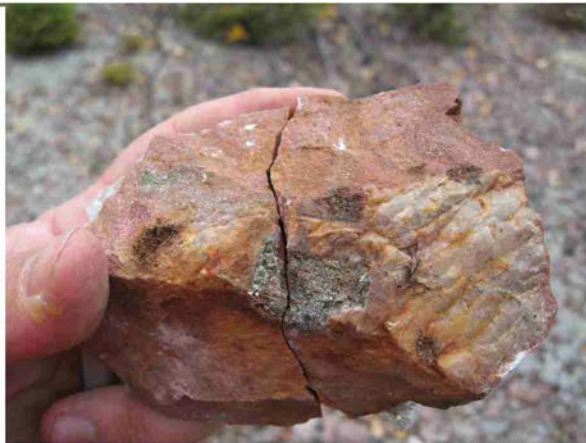
Fig. 9.13D Frontier adit dump: Cluster of fine grained pyrite on margin of quartz vein in f.g. pink granite?
