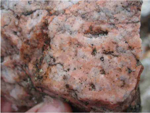
Fig. 9.11A Box mine area: pink Box granite with poorly defined crystal margins. Interpreted to be a result of late-stage metasomatism.
