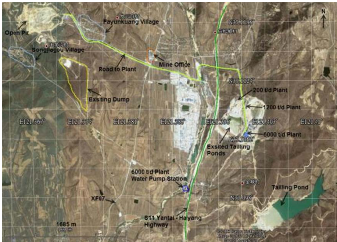
Figure 17-2: Mine Industrial Sites Lay-out
