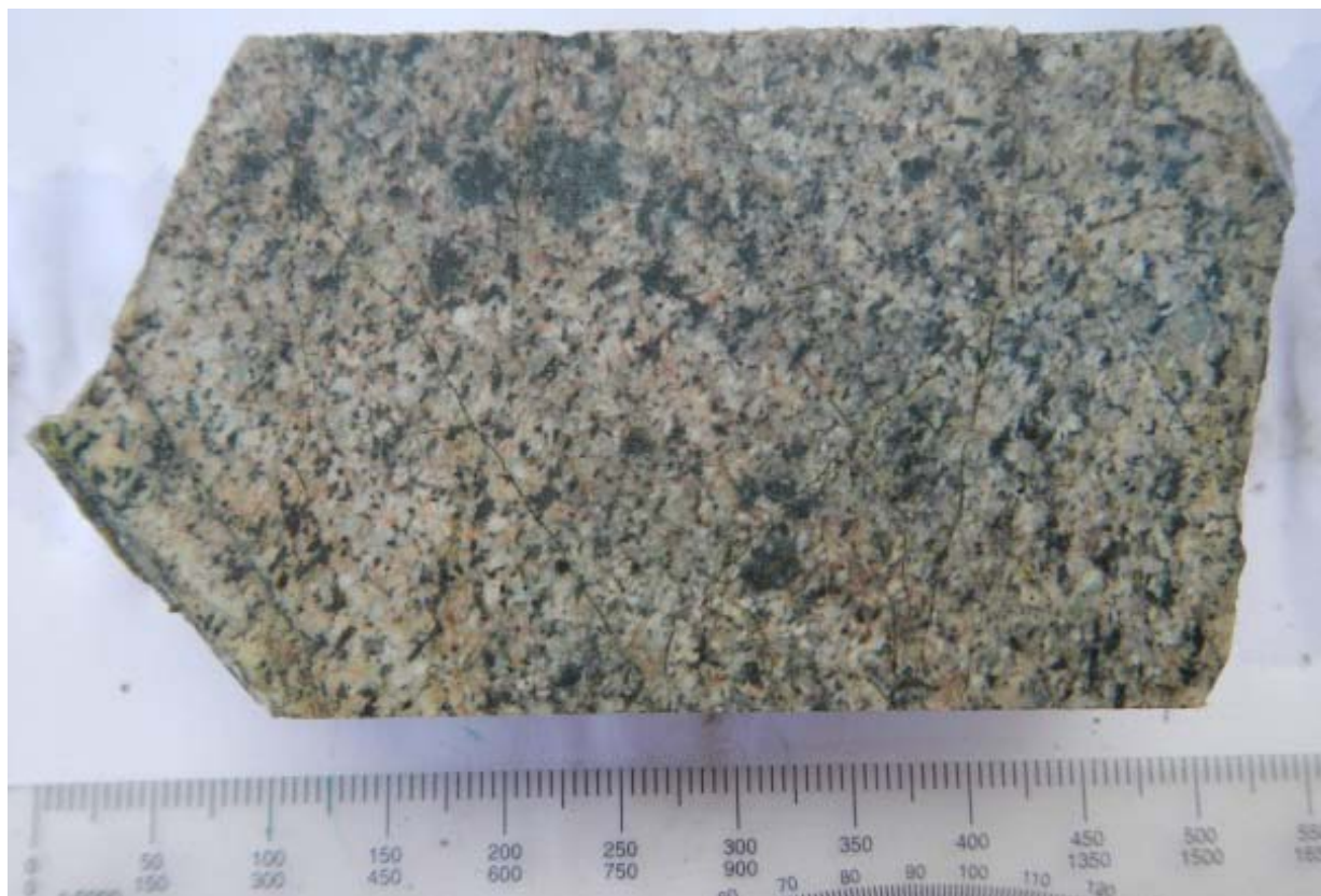
Figure 7-15: Potassium Feldspar Alteration in SLD
