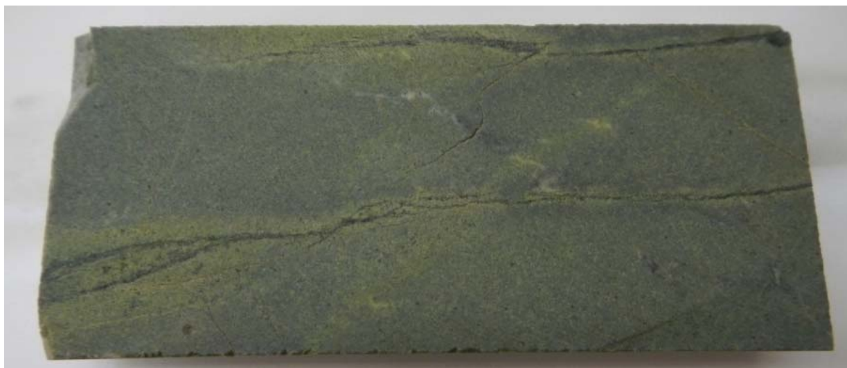
Figure 7-7: Mafic Volcanic (MAFV) with Epidote Alteration
