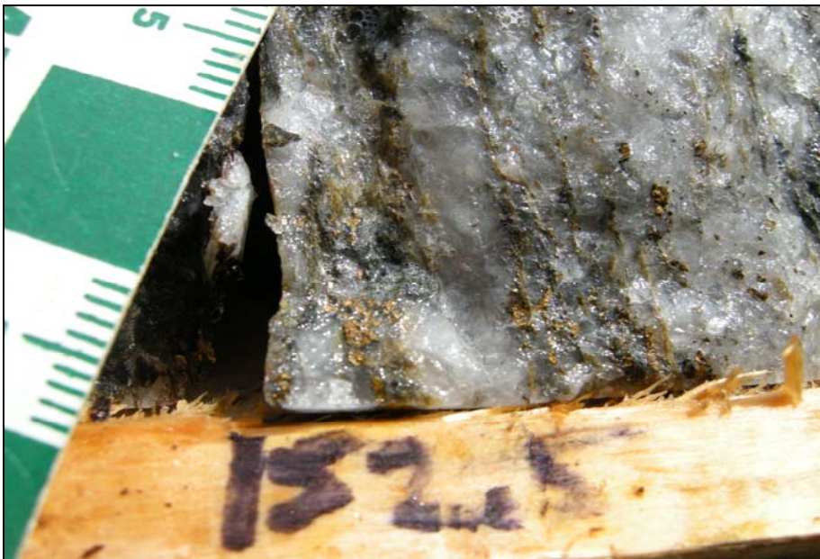
DDH 8-72 @ 152.5 ft along core: Sphalerite and pyrrhotite in quartz
