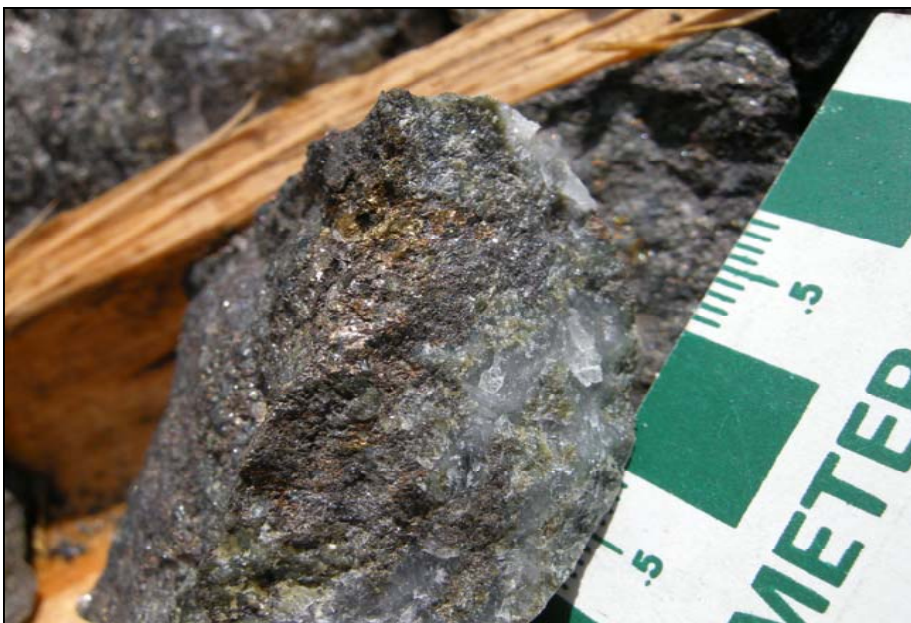
DDH 6-72 @ 355 ft along core: Sphalerite and pyrrhotite in quartz
