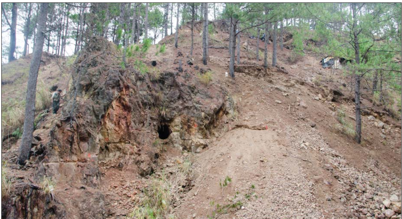
Figure 3: Small-scale artisanal workings in the north of the prospect. Artisanal miners drive small adits in the oxide zone and manually mine ore without compressors or blasting. Note also location of horizontal ECR channel samples in fore-ground.
