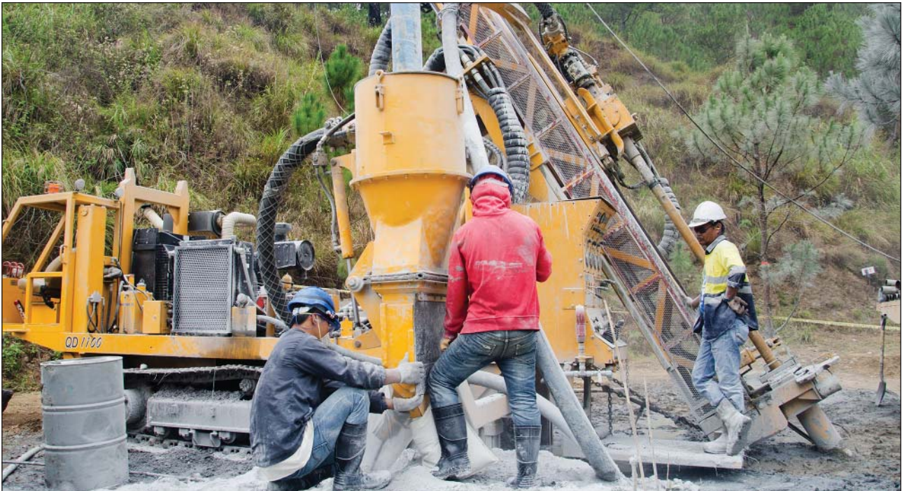
Figure 47: RC drilling at the Danglay prospect using an Edson 3000W drill rig fitted with a 4½ inch drop-face RC hammer. RC chips were sub-sampled using a Jones style riffle splitter.
