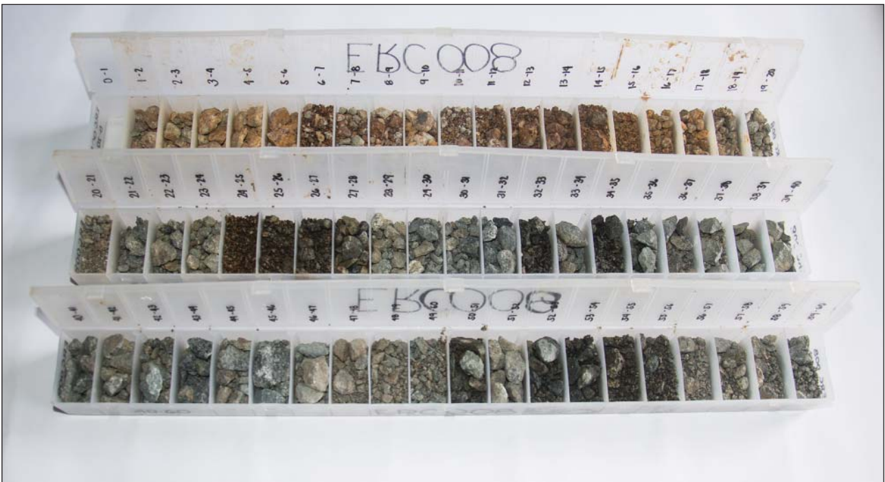
Figure 48: Example of the RC chips retained by ECR in industry standard RC chip trays. A representative sample of chips are taken from each sample interval.
