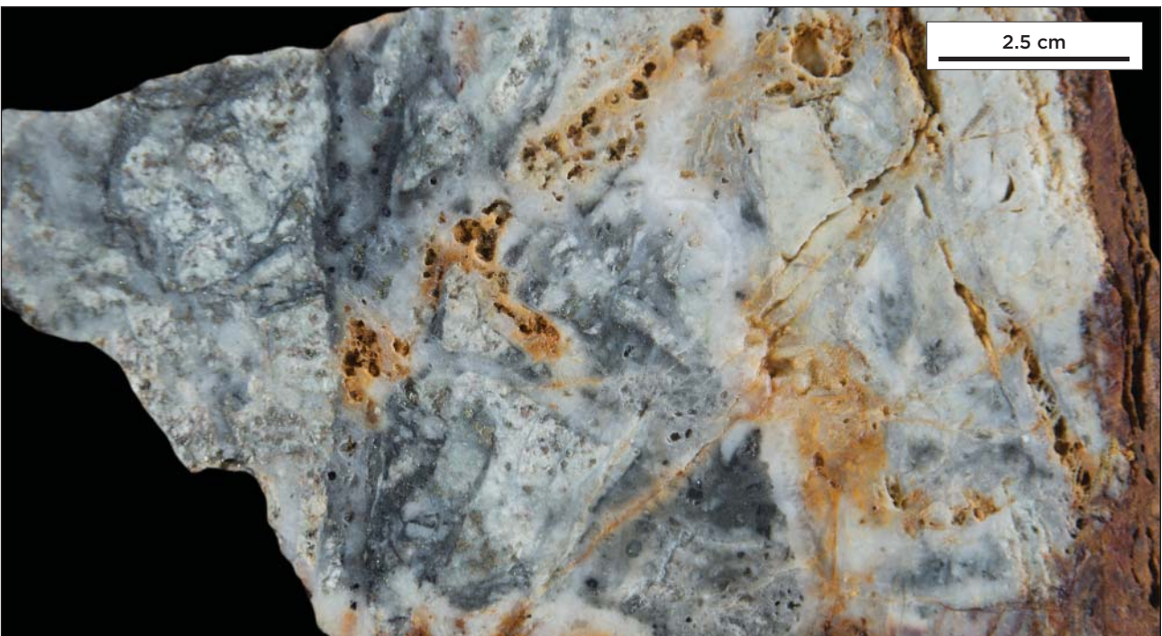
Figure 34: Strongly clay-silica minor pyrite altered diorite with pervasive stockwork of milk white to dark grey sulphidic quartz veinlets. Note patchy oxidation to limonite and vughs after sulphides. EAL sample ER01452 which assayed 34.68 g/t Au, 10.57 oz/t Ag and 0.22 % Pb.
