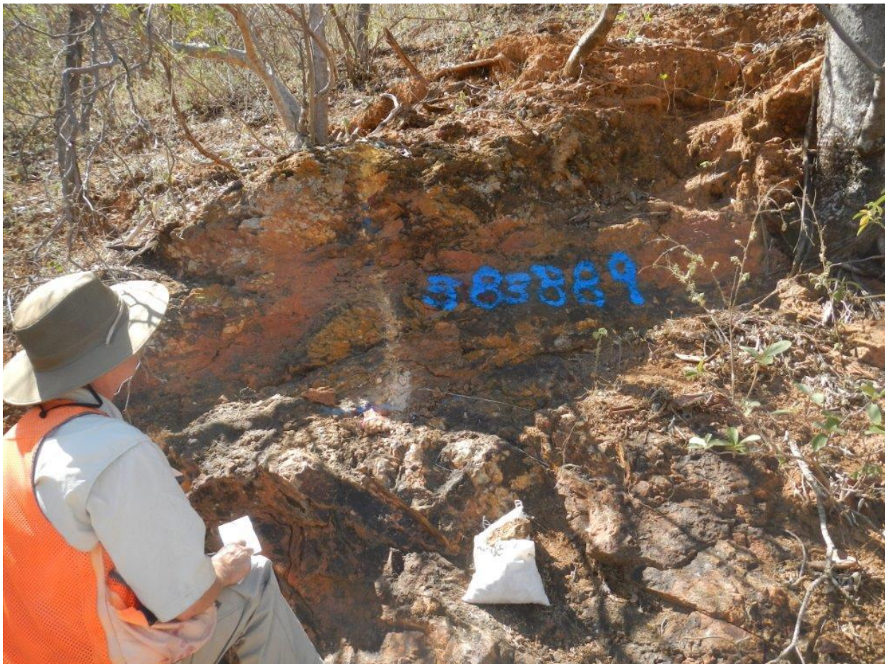
Figure 15. Chip channel sample 383889 near the middle of the Terrero area, 1.1 m @ 0.257 g/t Au, 557 g/t Ag, 13950 ppm Pb. This sample was not in a mined area and the outcrop was not particularly noteworthy compared to adjacent outcrops.
