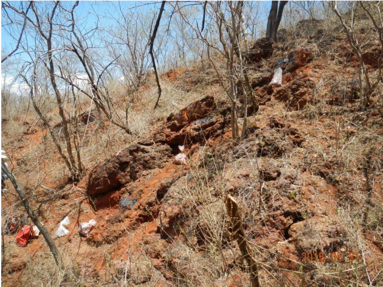
Figure 19. Consecutive samples 383946, 383947 and 383978 totaling 4.65 m with a weighted average values of 0.072 g/t Au, 3.55 g/t Ag, 60 ppm Cu, 1100 ppm Pb, 80 ppm Zn. The 4.65 m is nearly perpendicular to layering and is believed to represent true stratigraphic thickness.
