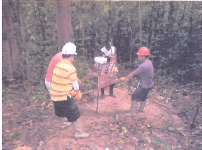
Plate 3. Power Auger Sampling
