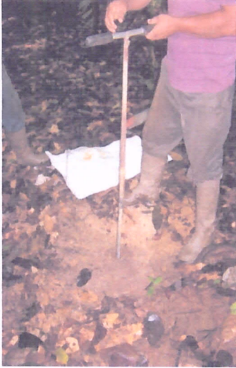
Plate 2. Hand Auger Sampling
